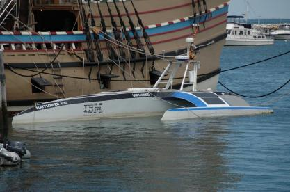
data analyzing devices. Radar scans for 2.5 nautical miles while cameras search for visible ships and hazards. An Automatic identification system provides data on approaching vessels. GPS provides location, speed and course data to help the Mayflower 400 navigate. Sensors monitor water depth and ocean conditions.
