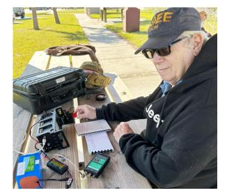
I, Ron, N9EE set up my IC705 with T1 tuner and 20 ft portable flag pole with my 40m OCF dipole.
