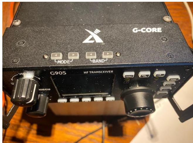
On the top of the radio are buttons to select the mode (CW, CWR, AM, LSB and USB) and the band (160-10 meters).
