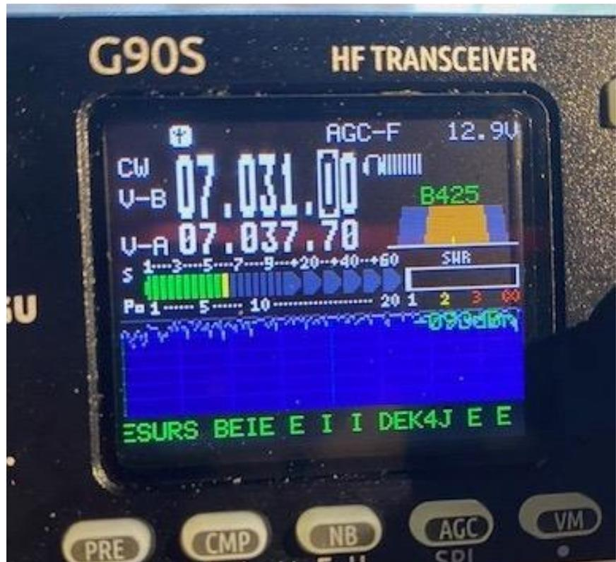
After 14 days, I feel comfortable with the controls and menus, although I do refer to the manual to learn more. The G90S has a built in Morse decoder. I have played around with it and although it is quirky, it does work in a fashion—for example, it frequently translates I as two Es. The manual is available at <http://www.connectsystems.com/products/top/radios/G90/G-90-Manual.pdf>
