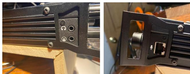
The sides have connections for the headphones and microphone and firmware updates for the detachable front panel.
