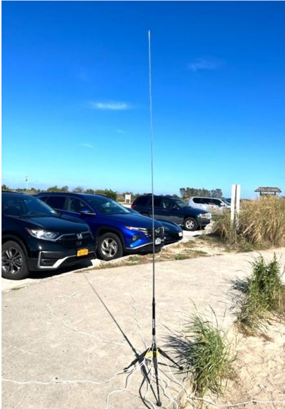
Walt W2TE and Tom KA2D: IC 7300 to a vertical jackite pole and they worked 10m and got as far as Venezuela
