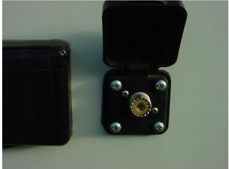
Modified cable input jack now sports a new connector
