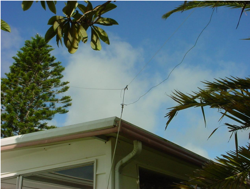
The feed point with 25' of RG58 connected, looking up to the NW
