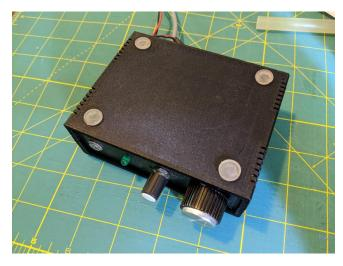
soft glues work well too. However, I advise against epoxies or other hard glues that might be difficult to remove should the glue wafers need replacing.
