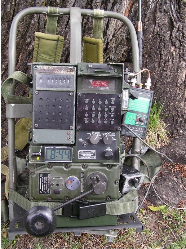
"10 Watter" on the ALICE pack with a small battery, the hand crank generator, and the T-1 tuner.
