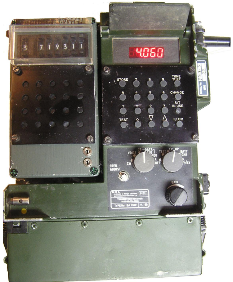
Front of the case. The display shows '4.060,' which is 14,060.0 for the 20 meter version.
