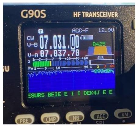
After 14 days, I feel comfortable with the controls and menus, although I do refer to the manual to learn more. The G90S has a built in Morse decoder. I have played around with it and although it is quirky, it does work in a fashion—for example, it frequently translates I as two Es. The manual is available at <a href="http://www.connectsystems.com/products/top/radios/G90/G-90-Manual.pdf">http://www.connectsystems.com/products/top/radios/G90/G-90-Manual.pdf</a>
