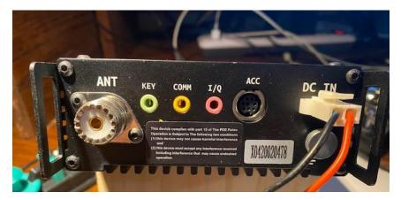
The back has connections for the antenna, keys (straight and paddle), various interfaces for firmware updates, computer control and power (Tamiya connector).
