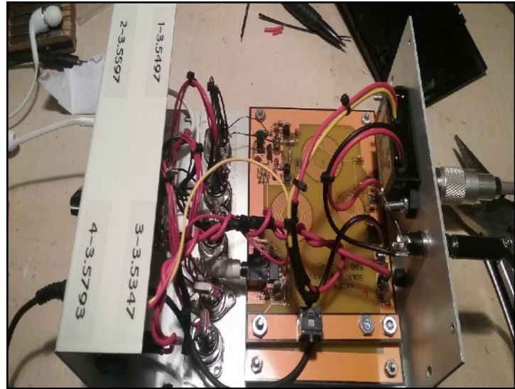
Cricket 80-A showing Buck Converter, and wiring layout
