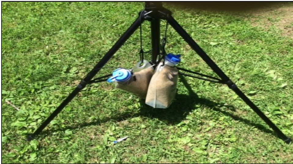
A useful addition to a Buddipole - inexpensive plastic canteens filled with sand. (The canteens can be found on Amazon.)
