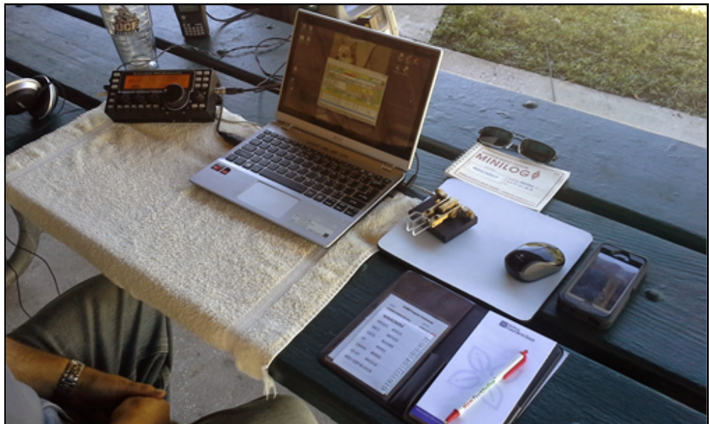
WB4OMM's PORTABLE SETUP - (from L to R) – Bose Headphones, KX- 3 Transceiver, Acer Laptop (Win 8.1), Vibroplex Code Warrior Iambic Key, Wireless Mouse, iPhone (Hot Spot). This entire station, along with 50' of RG-58 coax, SuperAntenna, and EFW Antenna/Balun all fit into a standard backpack, along with writing pads, pens, Leatherman multi-tool, cables, a spare 12VDC gel cell battery. With 5W out, and interfaced to the laptop, all modes from 40M to 6M with about a 3 hour operating period with logging and internet.
