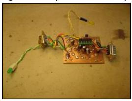
Step 2. Mount the five caps, one diode, three resistors, two LEDs, and connectors.
