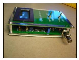
The two circuit boards make up the front panel as well as the case of the unit. I wanted some more protection from shorting out the circuit, so I cut a piece of posterboard and installed it on the bottom.
