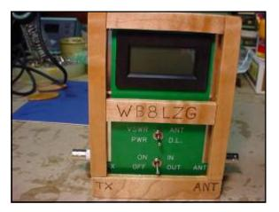
It took a bit of cutting, sanding, and a coat of varnish, but the meter now rests in its own wooden box. As a final touch, I personalized the box by wood burning the ports and my call. Now it sits proudly in the shack amongst the QRP gear. The bottom is removable to allow battery access, and with the BNC to RCA adapters removed, it is fairly compact. It is a FB addition to my shack.
