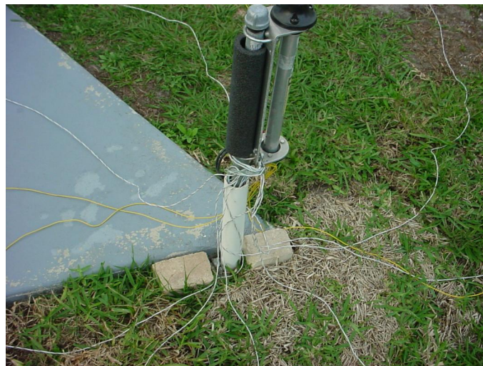
Close-up of 5BTV feed point with extra radials attached
