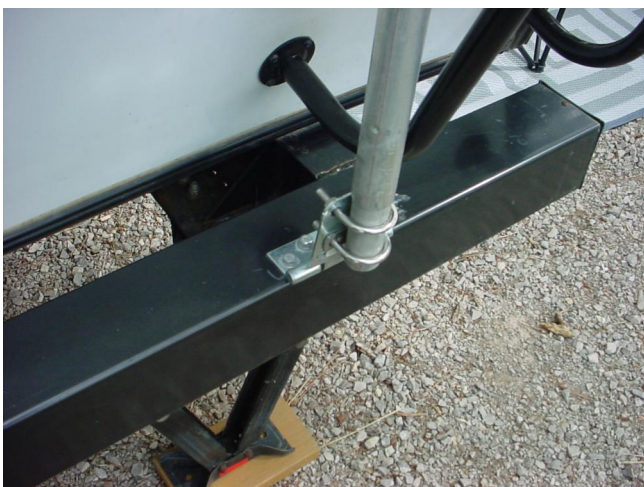
Bumper mounted fence hinge to secure bottom of mast
