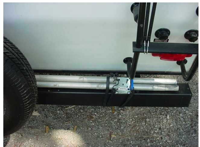
Mast secured to bumper for travel with bungee cords
