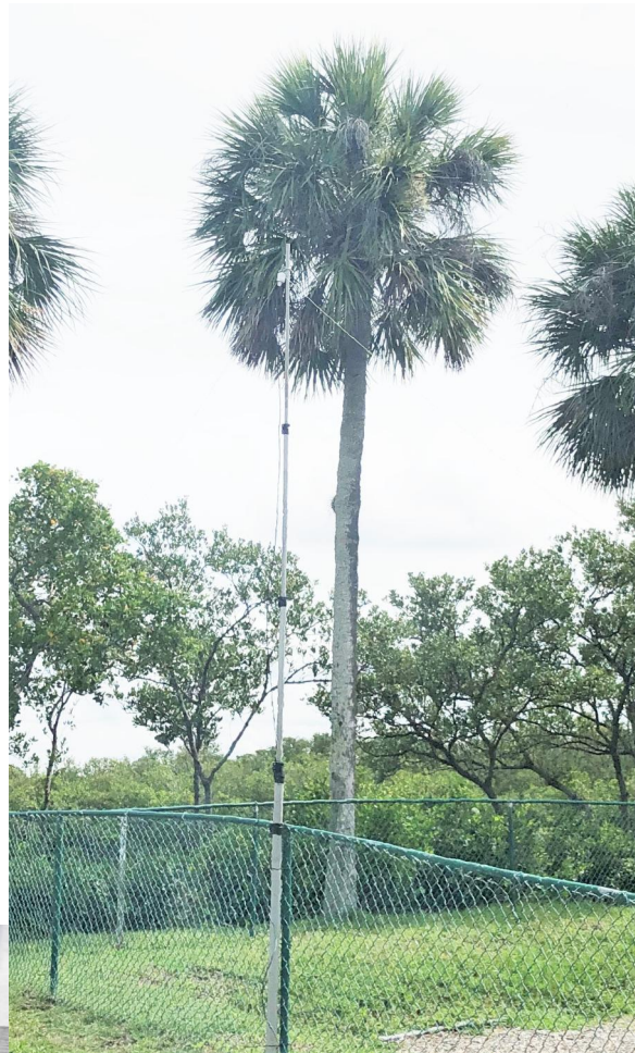
Dan's dipole on MFJ push up pole
