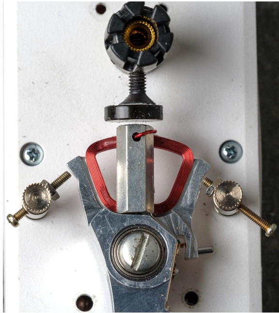
Fig. 4: Magnet and contact detail
