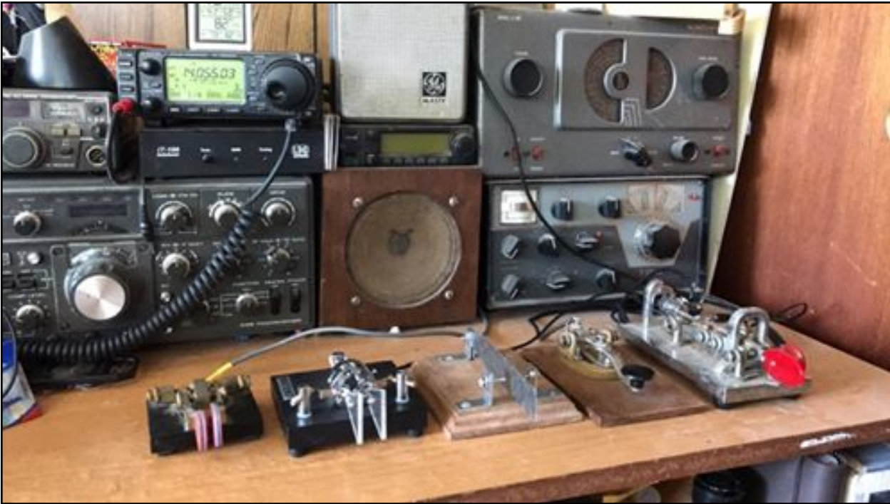
The lineup, L to R: Vibroplex Code Warrior Jr, Bencher BY-1, Homebrew Cootie, Generic Straight Key, Vibroplex Bug c. 1930's
