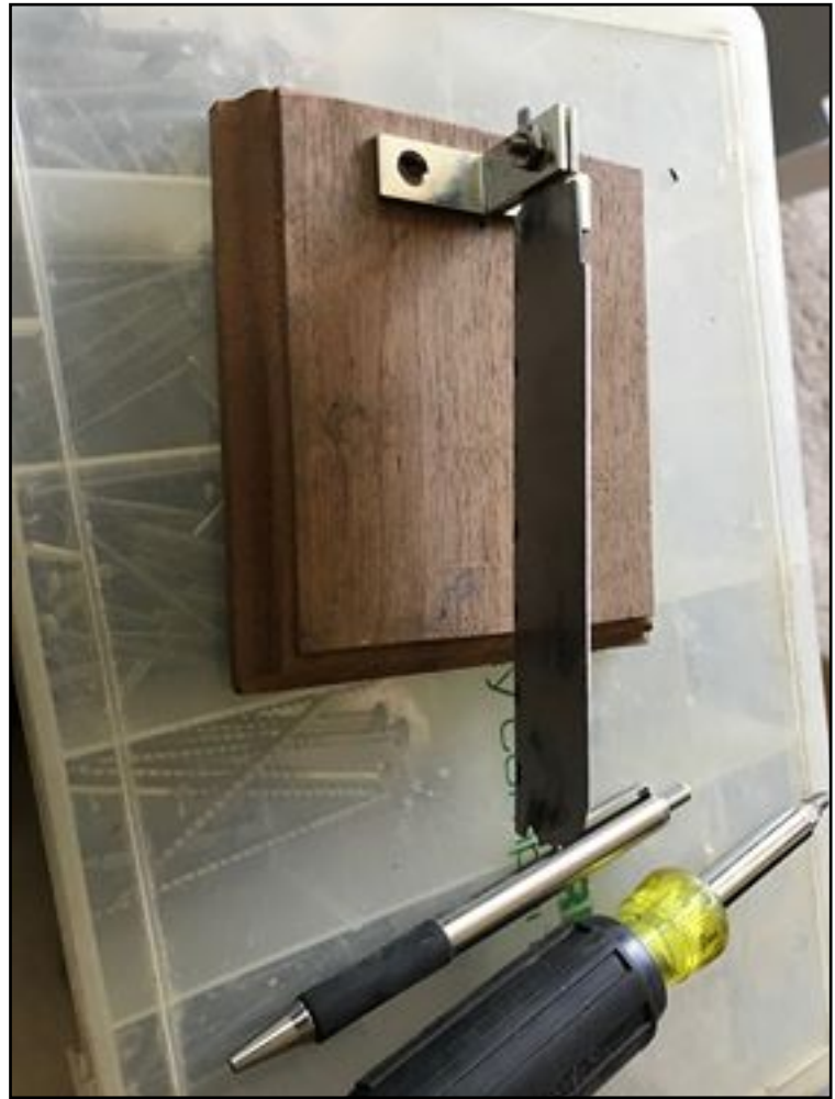
Base, support brackets, and de-toothed Sawzall blade.
