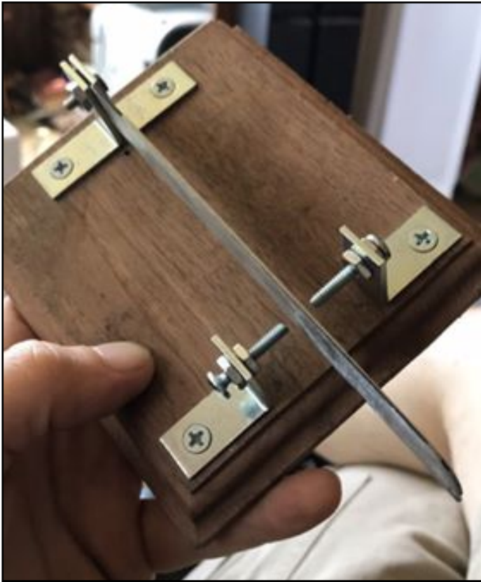
Machine screw terminals installed.
