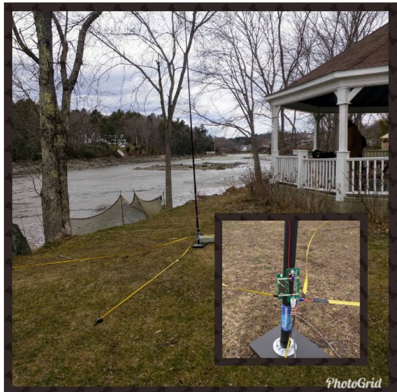
QRPguys Tri-Band vertical with tape measure radials.
