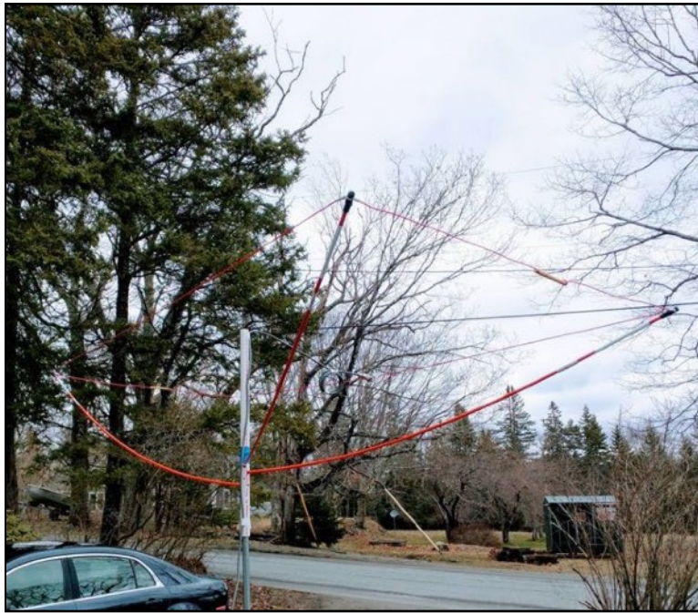
First set up of the portable 6 meter Moxon
